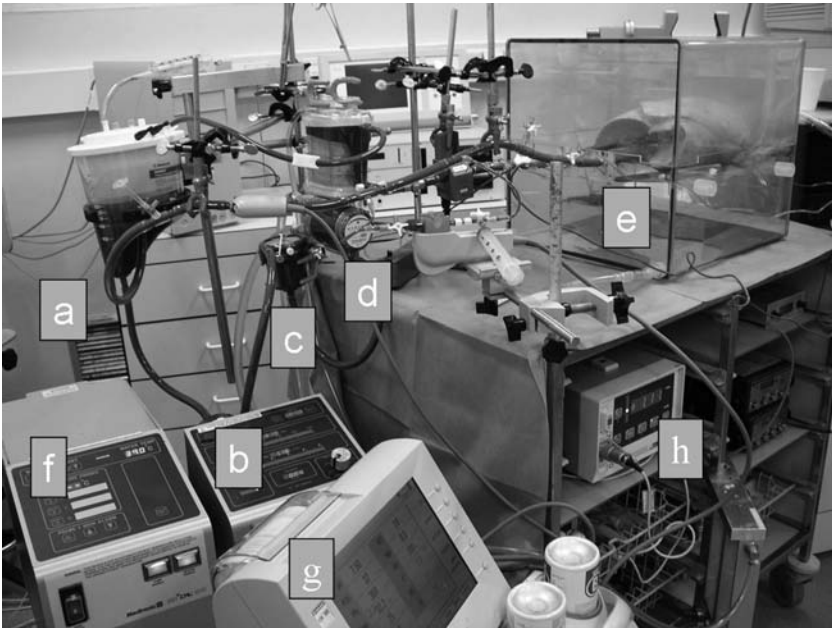
Figure 1 (See color insert) Isolated reperfusion circuit for ex vivo assessment of pulmonary grafts. From the hard shell reservoir (a) the perfusate is recirculated by a centrifugal pump (b) passing a leukocyte filter (c) and a membrane oxygenator (d) before entering the lung block (e). The heater/cooler (f) is connected to the membrane gas exchanger. Blood gases and pulmonary artery flow are continuously measured using an inline blood gas analyzer (g) and an electromagnetic flow meter (h), respectively.
